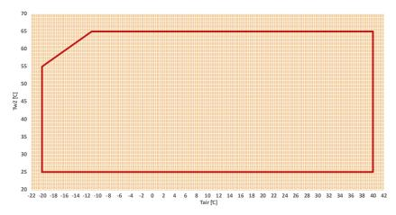
EvitecH heat pumps and are designed for heating or cooling the water to be used in air-conditioning systems for residential, commercial or industrial use. The execution with injection steam compressors (EvitecH) guarantees the production of hot water at high temperatures even in very hard outdoor conditions (up to -20°C).
