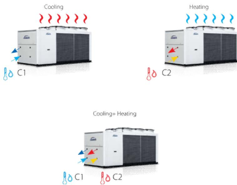
Operating modes available for an LCP P unit which interfaces with a 4-pipe air conditioning system.
