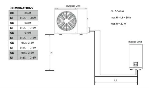
The maximum total length of the pipes for the connection between the outdoor unit and the indoor unit is 30 meters. The maximum difference in height allowed between the two units is instead 20 metres.
