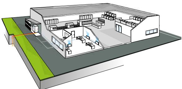
The possibility of keeping the evaporator indoors means there is no need to add glycol to the water inside the system. In addition, you can keep all components requiring maintenance in an easily accessible room.
