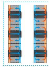
• the "In Rack" configuration, where a closed circuit is created between the rack cooler and the rack unit.
