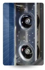
All models of the NRC range are factory-fitted with DX coils with hydrophilic treatment of the fins. The particular coating, combined with proper design of the air flow passage velocity, encourages condensate collection during the dehumidification process, thus avoiding water drops being dragged outside of the unit.
