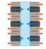
• the "In Row" in which cold air is released into the "cold aisle" to each rack cabinet and hot air is taken in by suction by the rack cooler from the surrounding environment.
